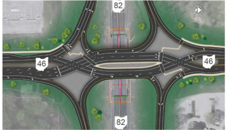
Proposed Diverging Diamond Interchange - Source: ODOT
